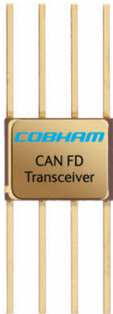
Cobham is using upscreening technologies and years of knowledge to create a radiation-hardened CAN bus network interface.
